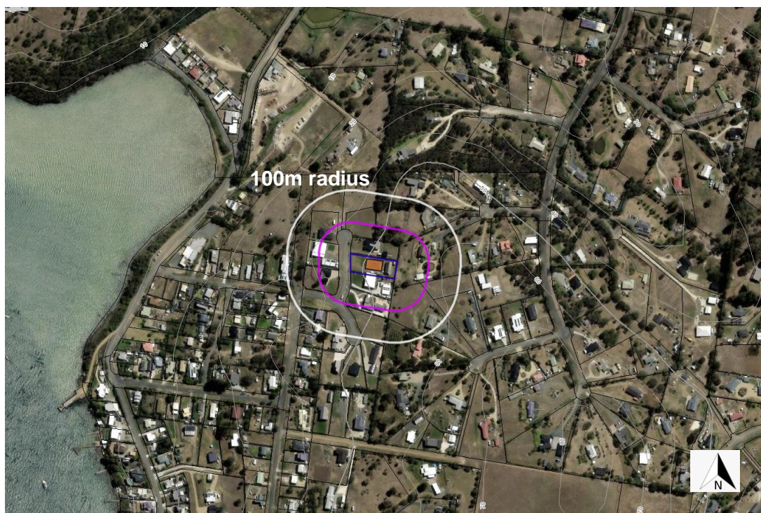
Figure 1: contoured listmap. www.thelist.tas.gov.au . Property in blue outline, proposed dwelling in orange and black. White outline is 100m from HMA, pink line 50m from HMA.
