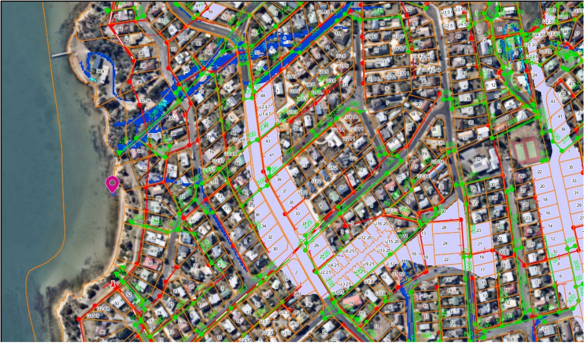
Figure 9 McKinly St Beach sewer in red; stormwater in green, flood risk and waterway shown
