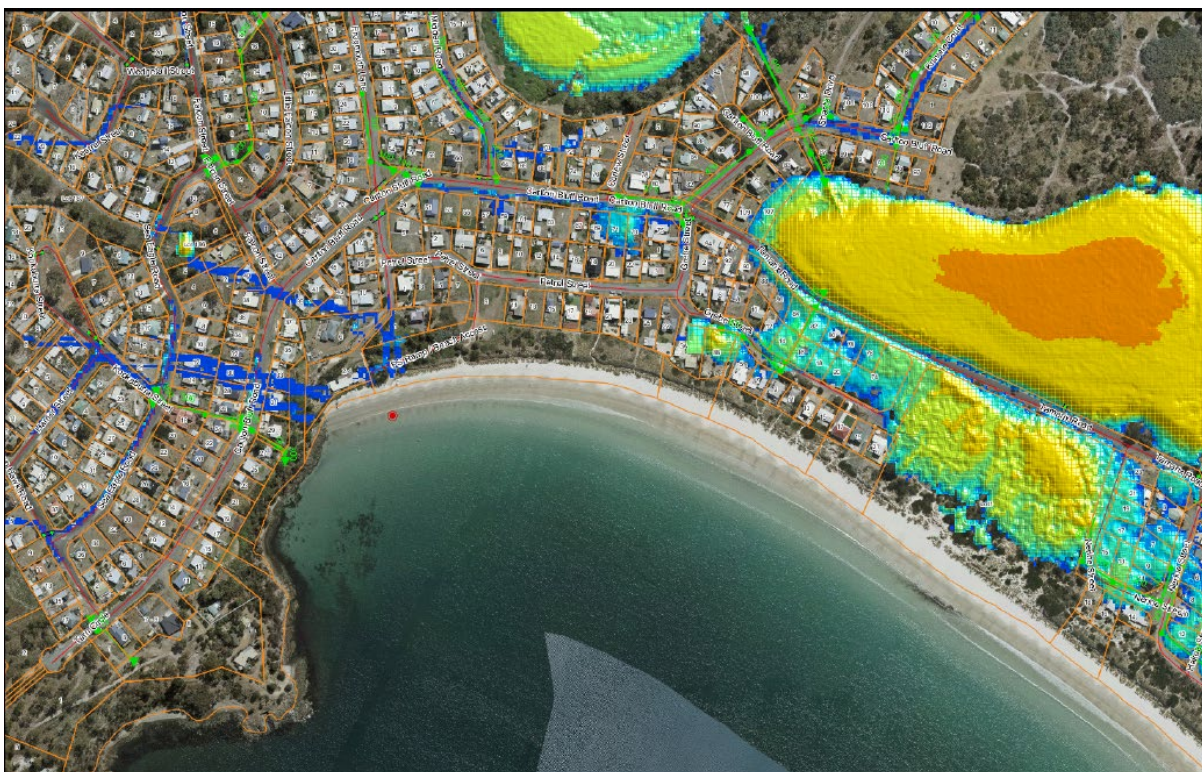
Figure 4 Primrose Sands Beach showing flood extent and stormwater infrastructure
