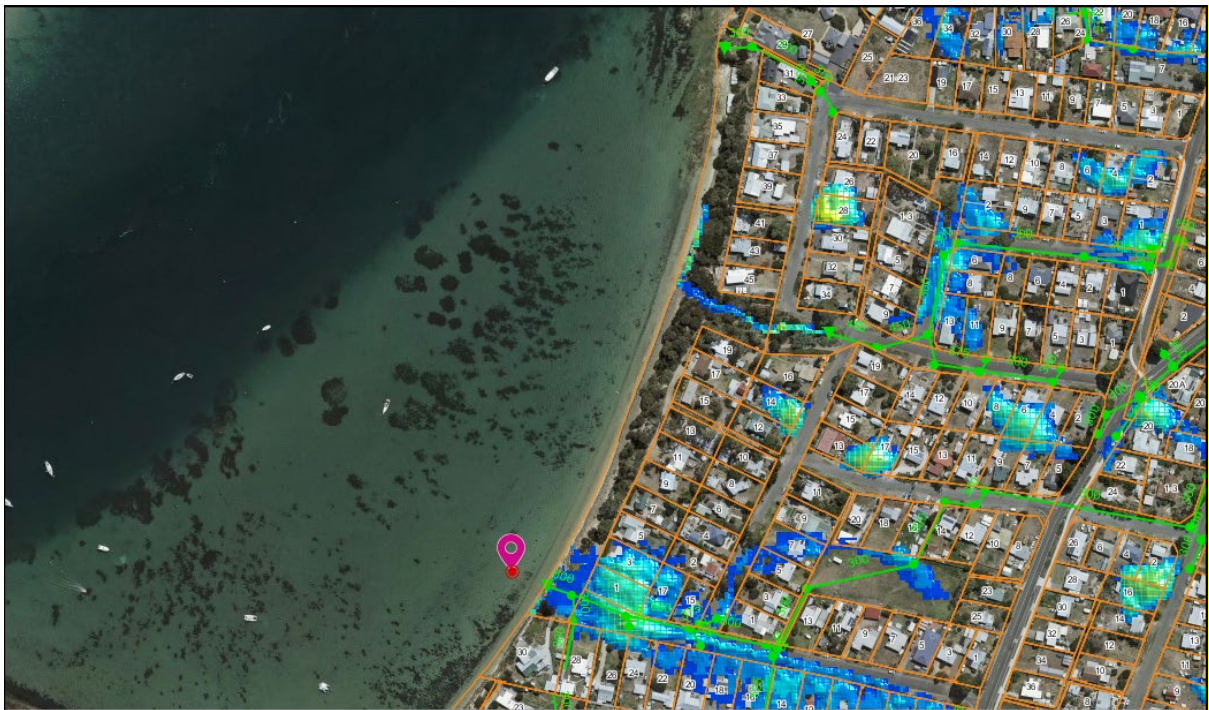
Figure 8 Tiger Head Beach @ 7th Ave showing flood extent and stormwater infrastructure
