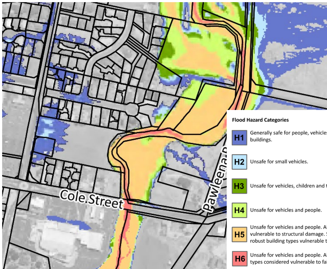
Figure 13. Flood hazard rating (Entura SSMP)
