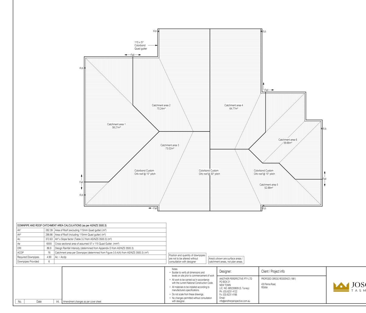
GUTTER OVERFLOW REQUIREMENTS as per N.C.C. Figure 7.4.6a: Minimum slot opening area of 1200 mm<sup>2</sup> per metre of gutter and the lower edge of the slots installed a minimum of 25 mm below the top of the fascia. The acceptable overflow capacity must be 0.5 L/s/m.
