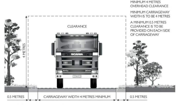
Figure 5 Carriageway width and clearance
