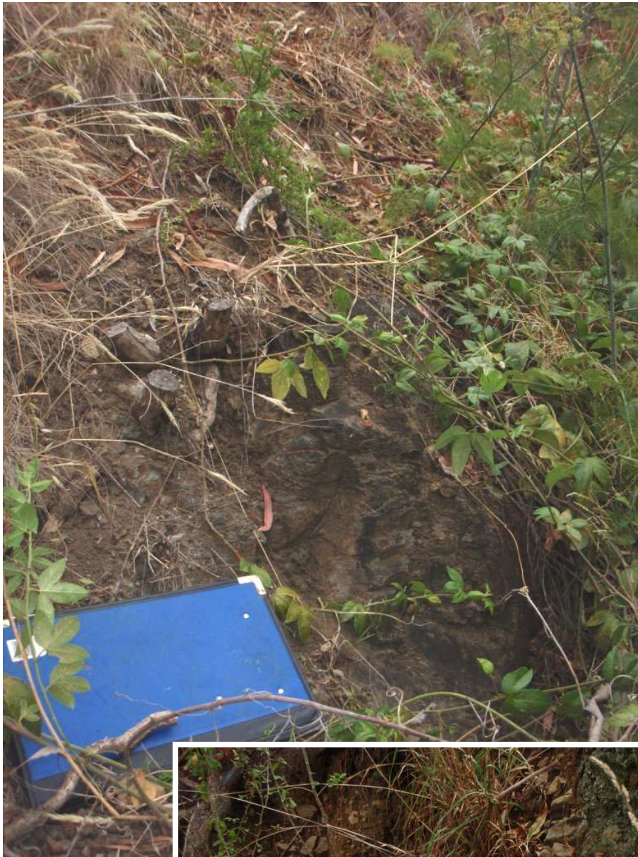
Plates 4 (left) and 5 (below). In-situ, strongly fractured Jurassic dolerite bedrock exposed in the banks of the intermittent creek along the northeastern boundary to 513 Shark Point Road.
