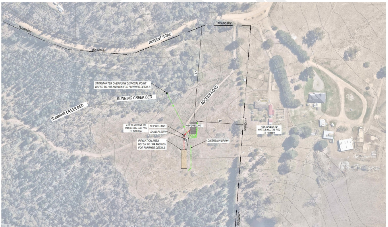
Figure 5: PROPOSED WASTEWATER SITE LAYOUT (OVERALL)
