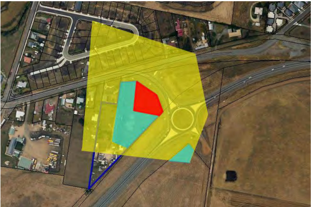
Figure 7: Site analysis. Subject site outlined in dark blue. All land within 100 m radius of the proposed childcare centre site (highlighted in red) is classified as either low threat or managed land (highlighted in yellow) and grassland (highlighted in blue). (source: The LIST, 17.05.2024).
