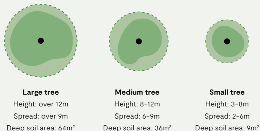
Fig 10. The approximate deep soil area required to support different sized trees at maturity.
