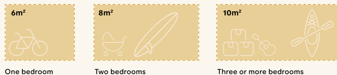
Fig 13. The recommended storage space to be provided for different sized dwellings. This is in addition to storage provided in kitchens, bathrooms and bedrooms.
