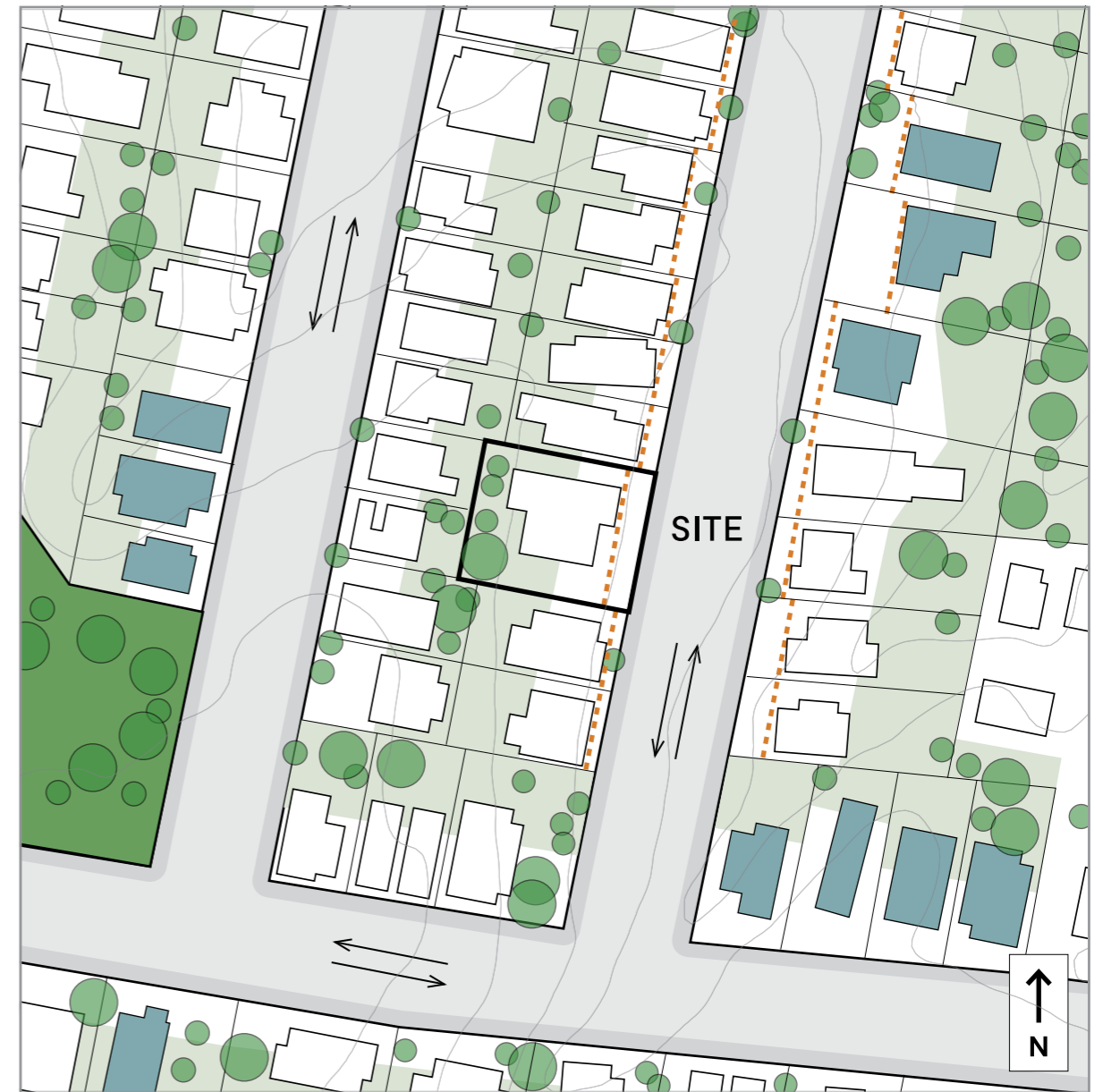
Fig 2. Context plan at the streetscape scale showing the surrounding built form, prevailing street setback, open spaces, and access patterns.
