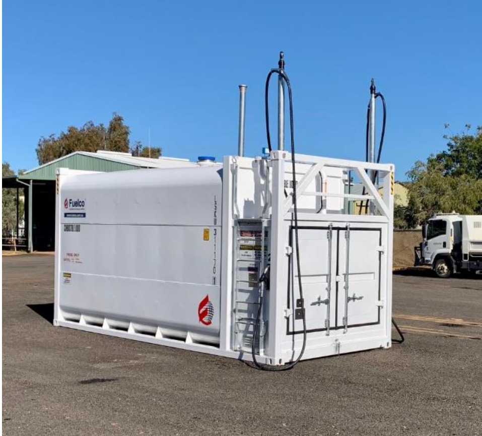
Figure 7: Self bunded fuel tank
