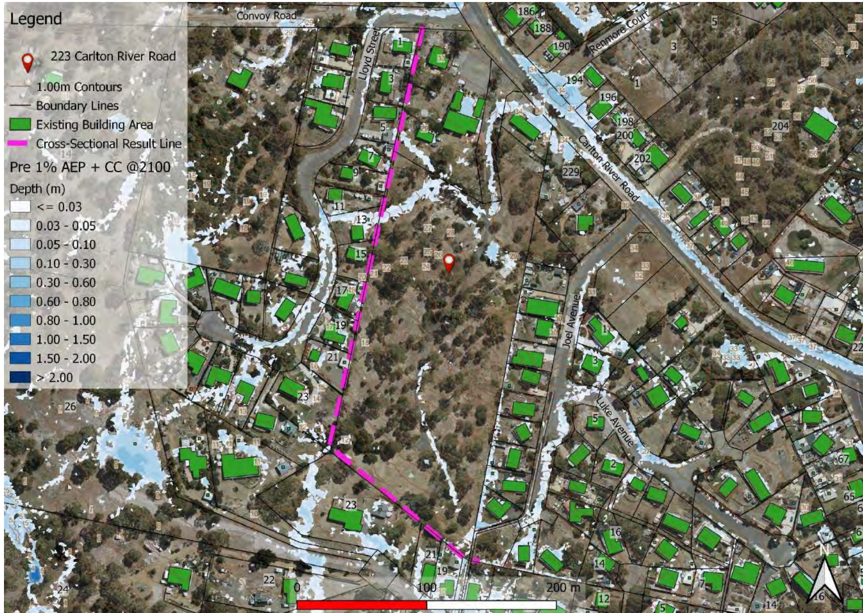
Figure 4. Pre-Development 1%+CC Flood Depths and extents
