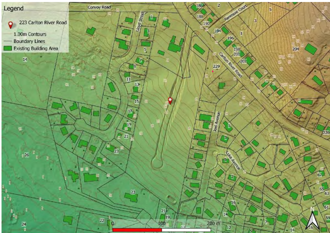
Figure 3. 1m DEM (hillshade) of 223 Carlton River Road, Carlton.
