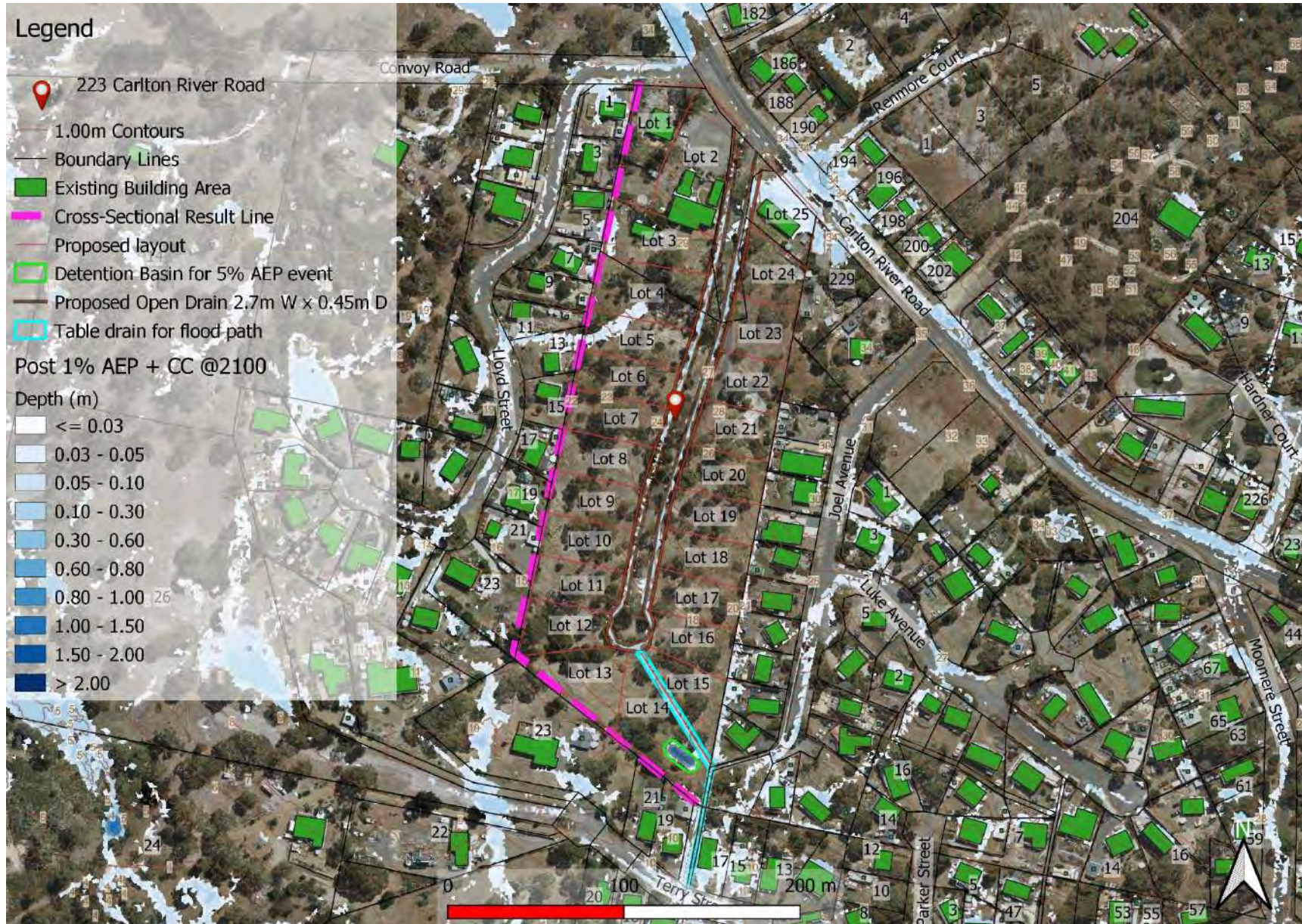
Figure 5. Post Development 1%+CC Flood Depth and extents
